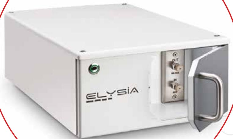
The Pomo is specially designed for radio flow monitoring of PET tracers. The detector represents the latest enhancements in flow detectors for radio HPLC.
