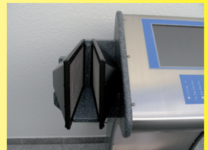
Fig. 4: Version with 2 detectors per hand, vertically mounted
